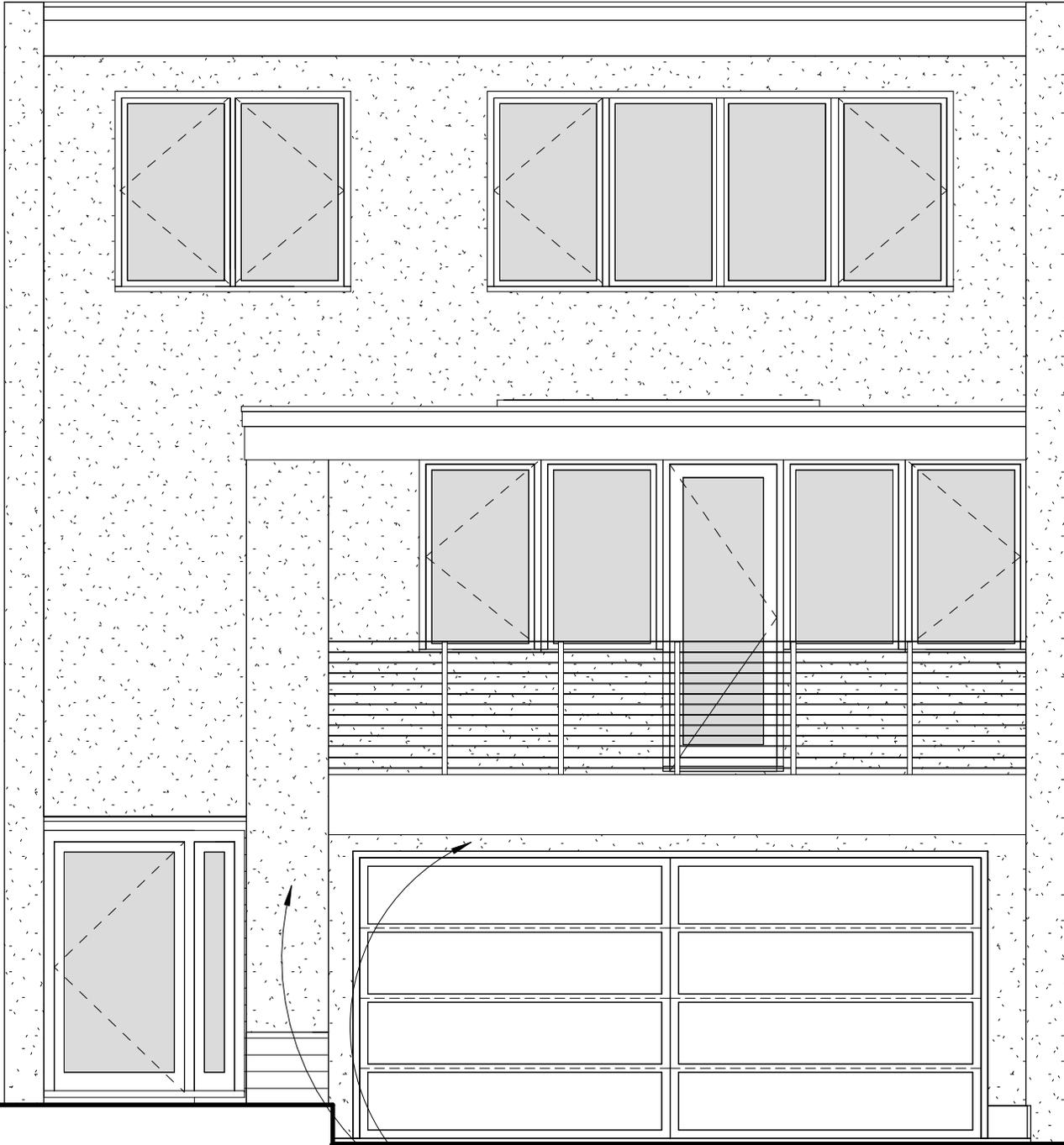
Cement plaster finish at new column and around garage door in lieu of cedar siding
